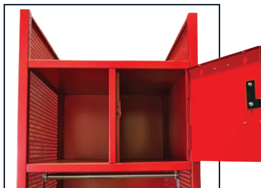
OPTIONAL SECURITY BOX USES TWO HEAVY-DUTY 13 GAUGE 7-KNUCKLE 3-1/2" HINGES AND A FINGER PULL PADLOCK HASP
